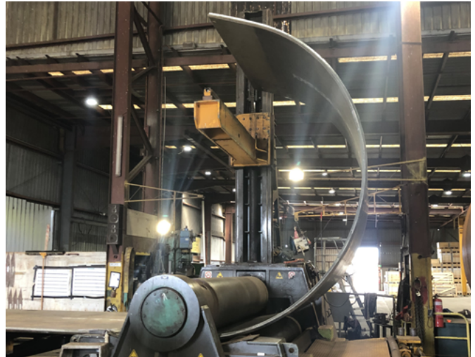
XLERPLATE® steel rolled for tower base plates - Nordex Mortlake Wind Farm
